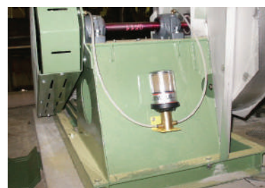
Food industry: lubrication of Solyvent Ventec ventilator bearings.
